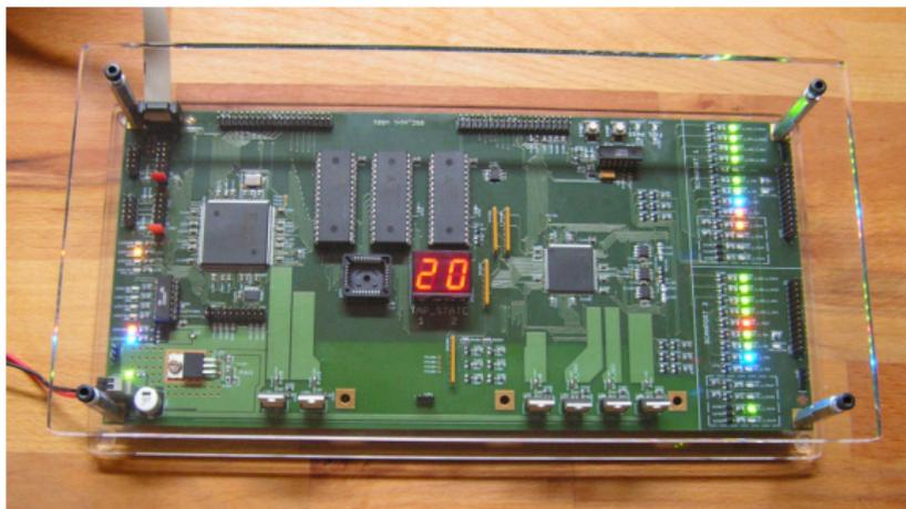
Figure 2: Boundary-Scan Controller (BSC)
