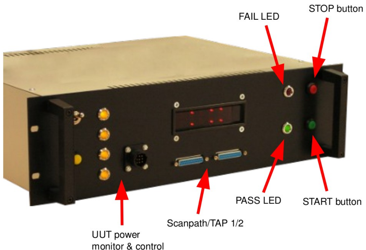
figure 8: BSC front panel
