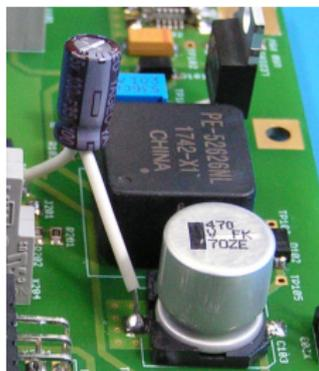
Figure 25: Kondensatoren THT/SMD
