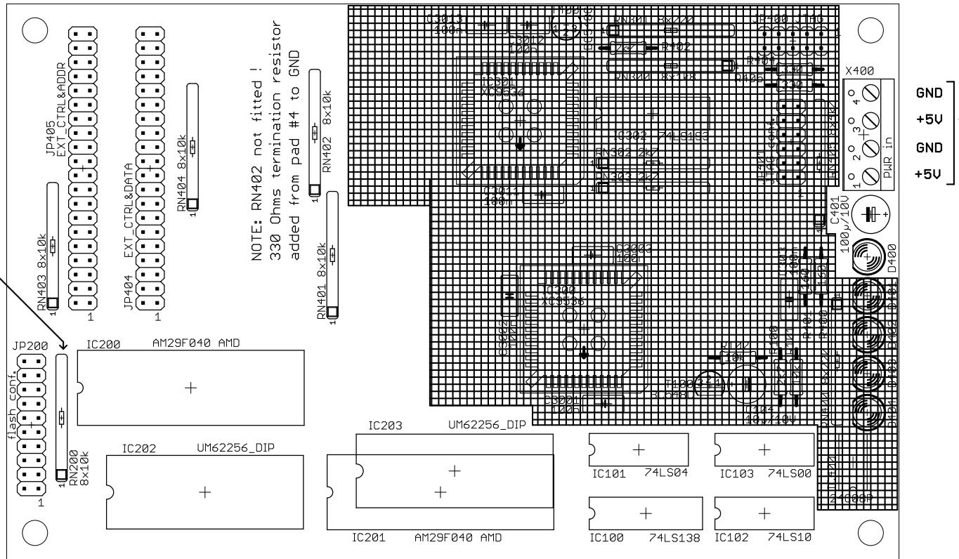
NOTE: pins 1 and 2 of IC200 and IC201 solder bridge.
